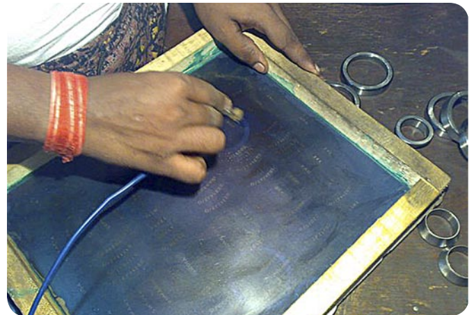
False markings are etched on bearings using silk screens such as this.
